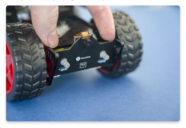
• Once in position, let the side panels close and secure the Headlights + Camera panel in place.
