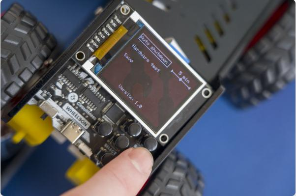
Once he is OFF, to switch him back on you can either press the RESET button or turn the switch off and then back on.
