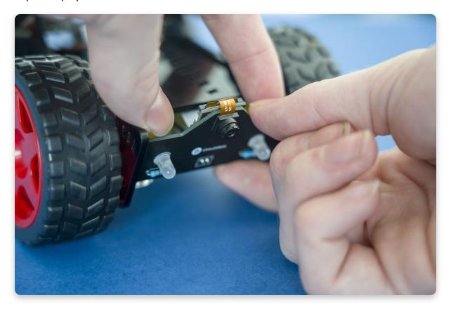
• Then move the Headlights + Camera panel into the forward-facing position with your hands, by slotting it into the top slot, as shown.
