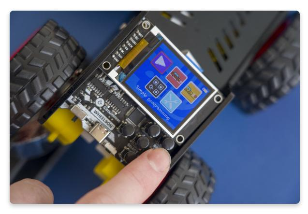
Navigate through Wheelson's menu by using the 4 directional buttons on Wheelson's control panel like in the photo.
