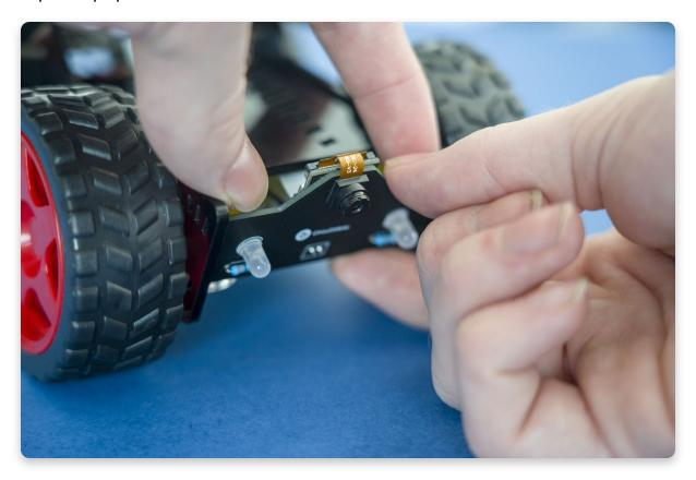
• Then move the Headlights + Camera panel into the forward-facing position with your hands, by slotting it into the top slot, as shown.
