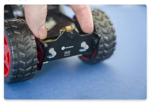
• Then move the Headlights + Camera panel into the lower-facing position with your hands, by slotting it into the bottom slot, as shown.
