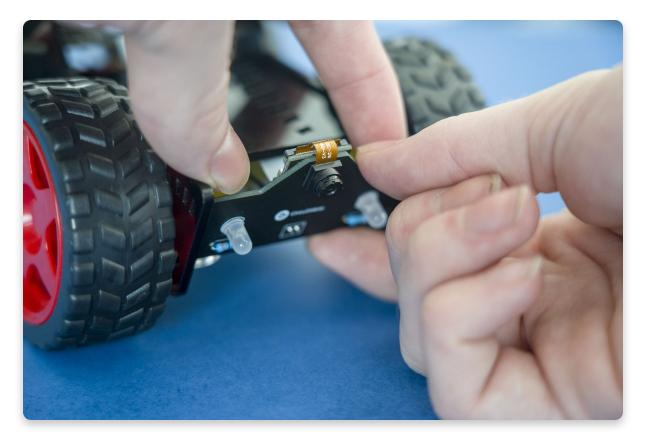
• Once in position, let the side panels close and secure the Headlights + Camera panel in place.
