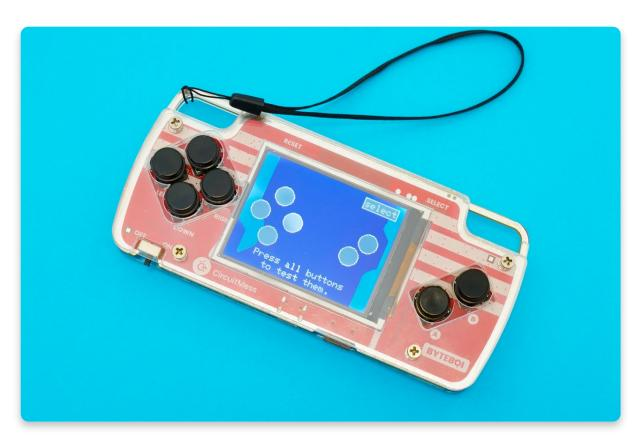
You should press all six of the ByteBoi's buttons you soldered a few moments ago. If the button is working properly, the circle representing that button should turn green. If one of the circles is not turning green, one of the buttons is not working. In that case, you should check the soldering joints on your buttons.
