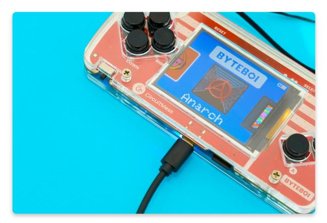
A battery icon on display will change colors while being charged. Also, you'll notice one LED lightening up left to the USB port as a sign of it being charged.
