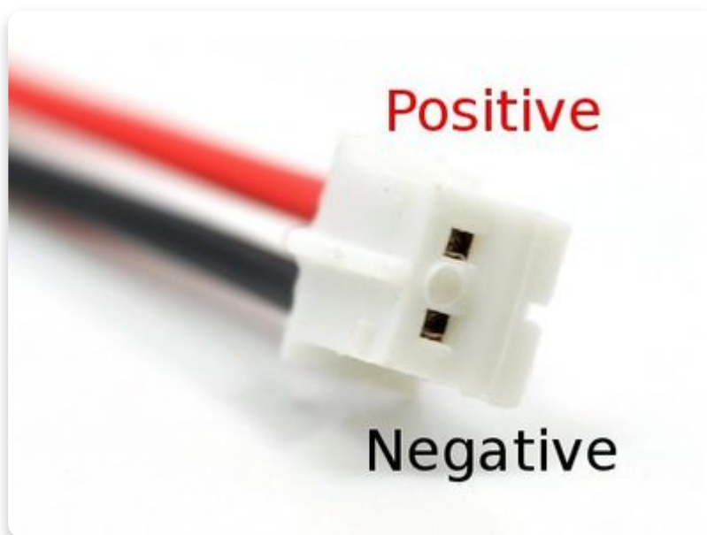
JST cable that connects the battery
