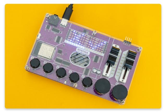
To exit the save menu, simply press any of the buttons, rotate or click the right encoder, or move one of the two sliders.
