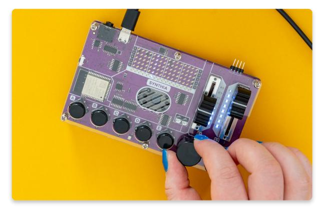
Rotate the right encoder to **select the effect** you wish to change, and then move the right slider to change the intensity of that effect. You can also use the left slider to **change the pitch of the sample**.
