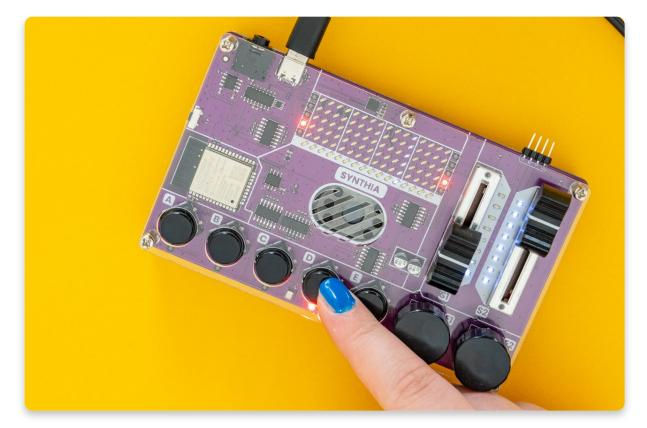
For example, we wanted to place the sample from the fourth pushbutton onto the sample. We had to click on the fourth pushbutton while being in the track to do that. The LED on the fourth row of the track lit up, indicating that a sample is placed in that position.
