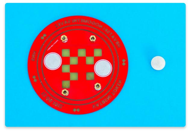
It is easiest to **place the battery board on a flat surface** and then place the batteries on the **board's silver circles**.
