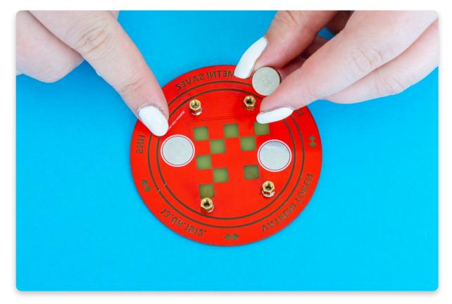
You can also take the other board from the kit (the one with + and - signs on it) and put it on top of the first board. This will give you an idea of how to properly place the batteries.
