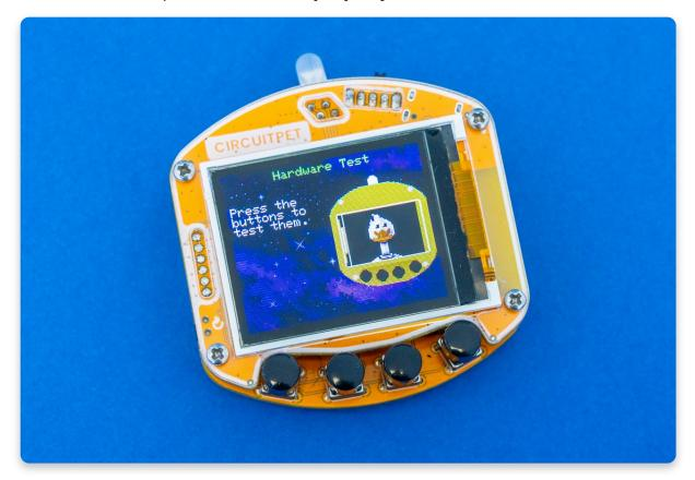
You should press all four of the CircuitPet's buttons you just soldered. If the button is working properly, the circle representing it should turn green. If one of
